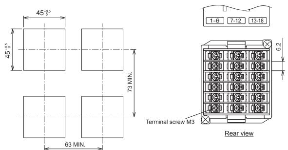
Terminal block is not attached to unused terminals (terminal 7 to 12) according to the model.
