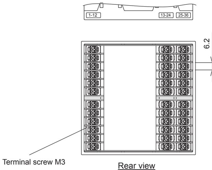
Terminal block is not attached to unused terminals (terminal 13 to 24) according to the model.
