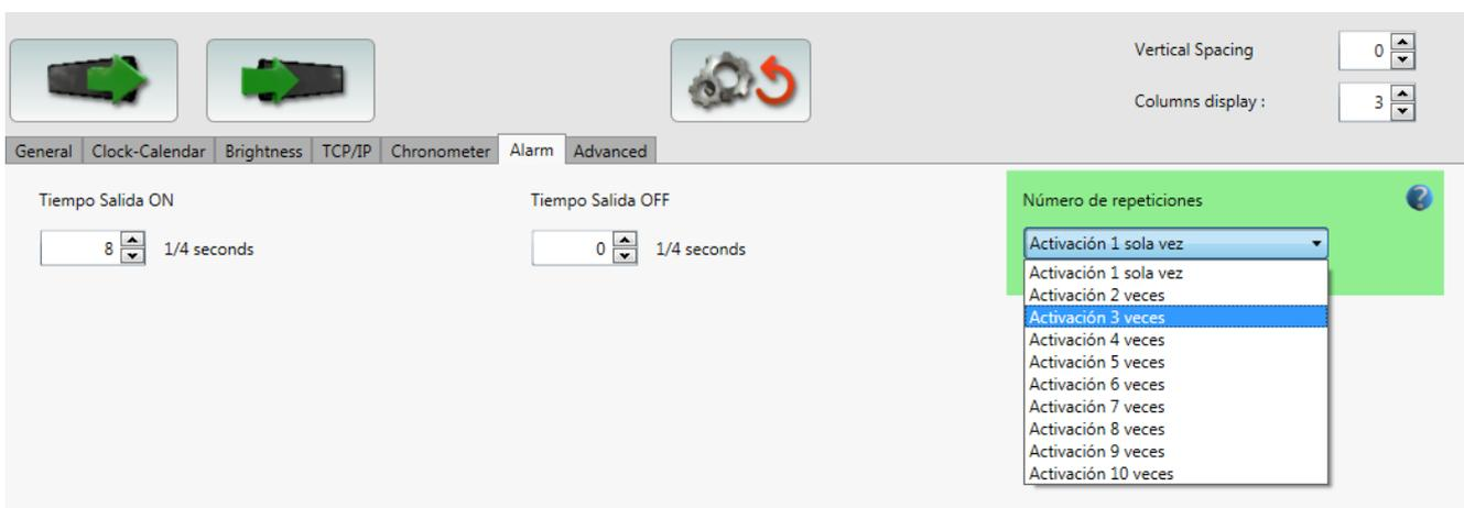
**ON Time:** Time in  $\frac{1}{4}$  seconds the output alarm stays ON.
