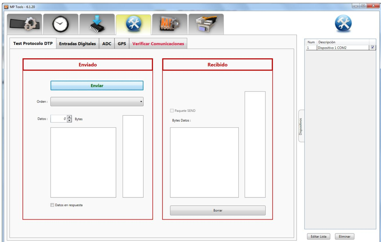
**Test Protocol DTPM:** Send orders in DTPM protocol which is the native protocol and read the response of the device. NOTE: Some orders can change or delete the device configuration. Only use with knowledge of the effects.
