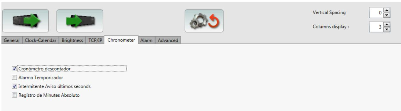
**Countdown chronometer:** Chronometer mode. If checked the chronometer works as countdown chronometer with the preselected Time 1, 2 or 3, If not as chronometer with final time (only with Time1).
