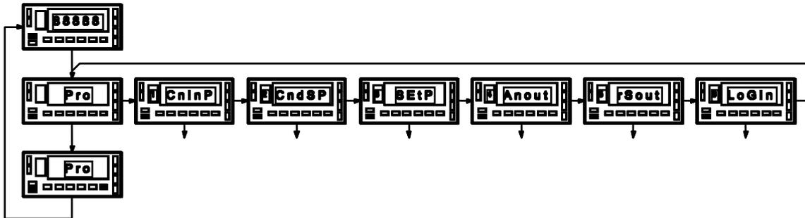
The programming instructions are composed by a general description and a series of step-by-step instructions to be followed sequentially. Each menu step is represented by an illustration of the display and keyboard module with indicators (display and LED's), reference [page number . figure number] and a text describing the action of each key at that step.
