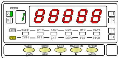
Figure 15.2 shows the indication corresponding to the entry level of the input select menu. The 8's represent any previously programmed input type but cannot be changed at this step.
