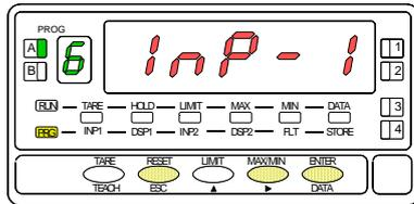
The figure 24.1 shows the indication (**InP-1**) corresponding to the configuration menu for the PIN 1 function. Press the **ENTER** key to accede this configuration.
