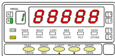
Figure 15.1 shows the entry level of the readout configuration menu where the 8's represent the previously programmed units and resolution but cannot be changed at this step. The following actions are available at this stage :
