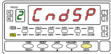
From the run mode, press **ENTER** to enter in the programming mode (the display shows -Pro- and the LED 'PROG' illuminates). Press **▶** twice to reach the stage represented in figure 17.1 corresponding to the display configuration module.
