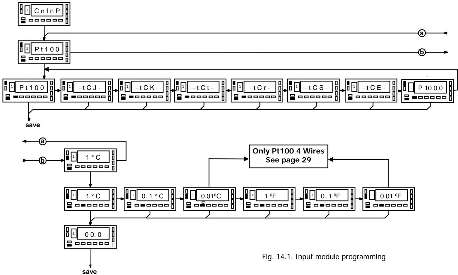
Fig. 14.1. Input module programming
