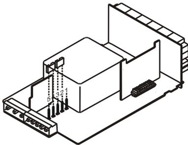
Fig. 10.2. Supply voltage 230 V or 48 V AC
