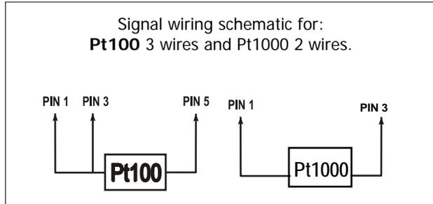
**Nota:** When using **Pt1000** sensor with 2 wires should be taken into account that every 0,385 ohms of wires resistance means a reading error of 0,1 °C.
