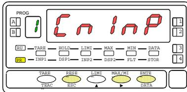
From the run mode, press **ENTER** to enter in the programming mode (the display shows -Pro- and the LED 'PROG' illuminates). Press **▶** to reach the stage represented in figure 14.1 corresponding to the input configuration module.
