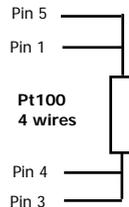
**Note:** If have been programmed Pt100 and 0.01° resolution, is mandatory to connect the sensor Pt100 with 4 wires, if not, the display shows error "-----"
