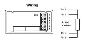
**Note:** If have been programmed Pt100 and 0.01° resolution, is mandatory to connect the sensor Pt100 with 4 wires, if not, the display shows error "-----"
