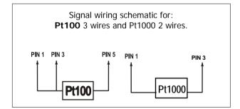
**Nota**: When using **Pt1000** sensor with 2 wires should be taken into account that every 0,385 ohms of wires resistance means a reading error of 0,1 °C.
