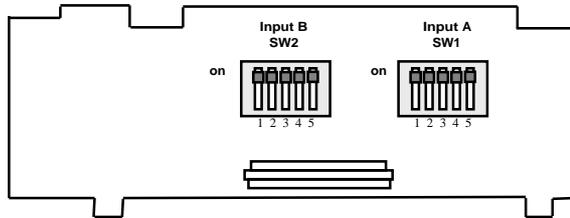
fig.11.1 : Solder side of input circuit board
