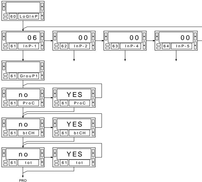
The logical functions are programmed on module '60 LoGInP'. There are 4 menus each one of them corresponds to an input of connector CN2 :
