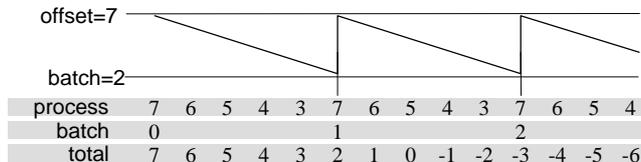
In bidirectional way, the function batch will be realized when an equal number of pieces is obtained to the programmed level, with independence of the previous evolutions of the counter.
