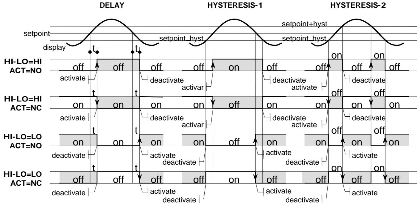
▲ : Activation edge of alarm where are done the setpoint functions (RESET, STOP, etc...) and where the relays make LATCH2
