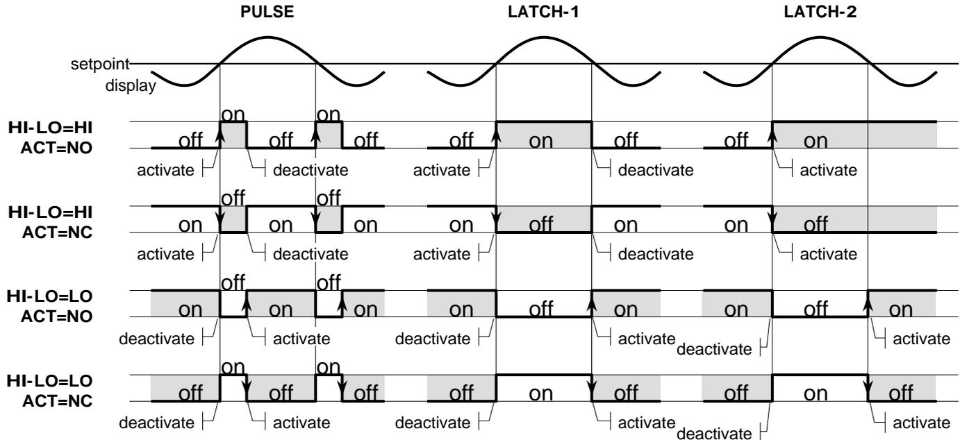
▲ : Activation edge of alarm where are done the setpoint functions (RESET, STOP, etc...) and where the relays make LATCH2
