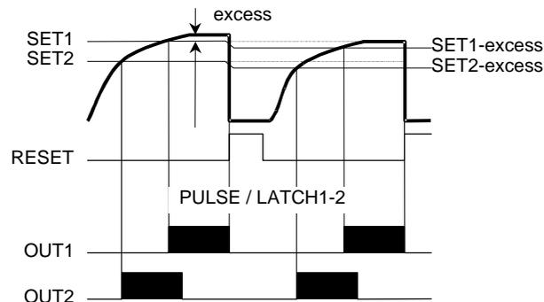
**SET1 = 100.0** (with function TRACK AUTO and way PULSE, the reset would be automatic on having come to 100.0)
