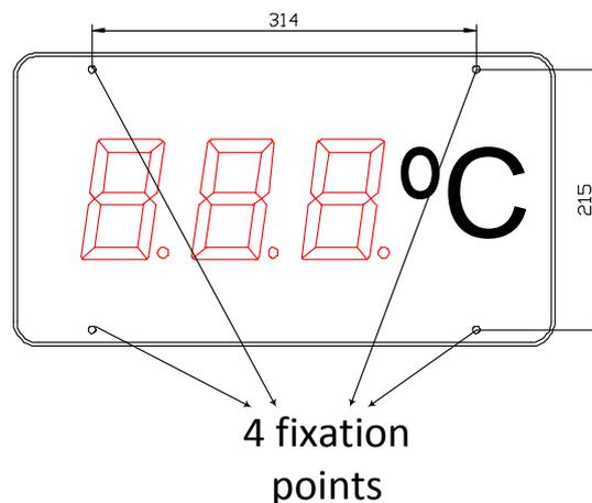
The DC-10 ST displays can be fixed to the wall in two ways:
