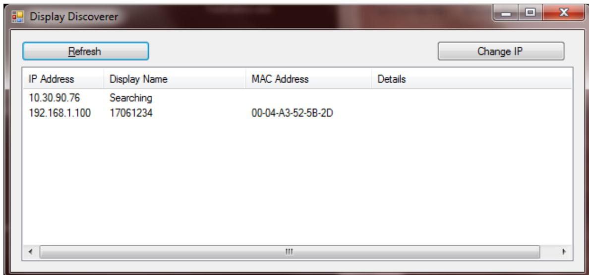
The first row shows the IP of the PC which is searching the displays and the second row a display we just have bought. As it is shown, the display has serial number 16601234 and the default IP is out of the range of the LAN. To change the IP address to a suitable one for our LAN, select the display and click the button "Change IP". When clicking this, a new window is opened where a new IP address can be typed.
