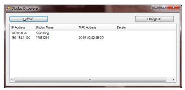
The first row shows the IP of the PC which is searching the displays and the second row a display we just have bought. As it is shown, the display has serial number 16601234 and the default IP is out of the range of the LAN. To change the IP address to a suitable one for our LAN, select the display and click the button "Change IP". When clicking this, a new window is opened where a new IP address can be tipped.
