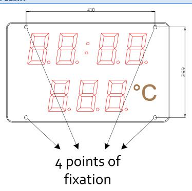
The DC-22 SRT displays can be fixed to the wall in two ways:
