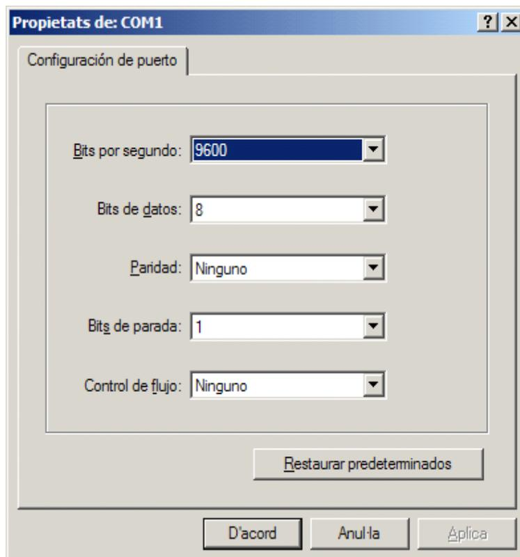
The attached Hyperterminal set up have been verified and work correctly, but any other set up may work also correctly.
