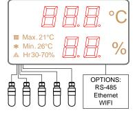
DC-21 displays are aesthetically identical to the DC-20 but do not have sensor. They must receive the data from RS-485, Ethernet or Wifi.
