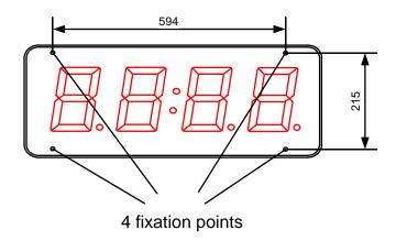
The DC-30 SR displays can be fixed to the wall in two ways:
