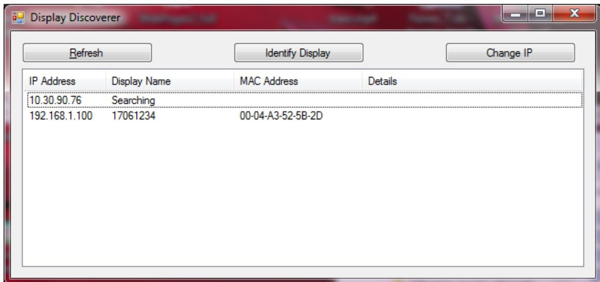
The first row shows the IP of the PC which is searching the displays and the second row a display we just have bought. As it is shown, the display has serial number 17061234 and the default IP is out of the range of the LAN. To change the IP address to a suitable one for our LAN, select the display and click the button "Change IP". When clicking this, a new window is opened where a new IP address can be typed.
