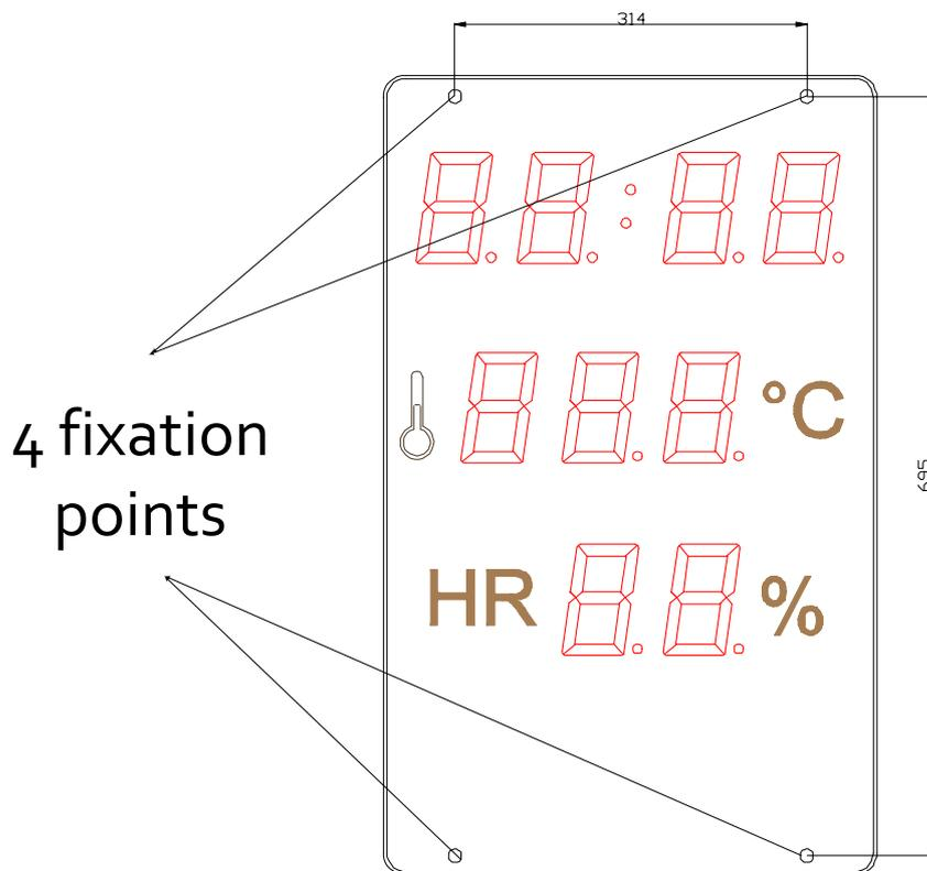
The DC-41 SRTHNE+2R/+4R displays can be fixed to the wall in two ways:
