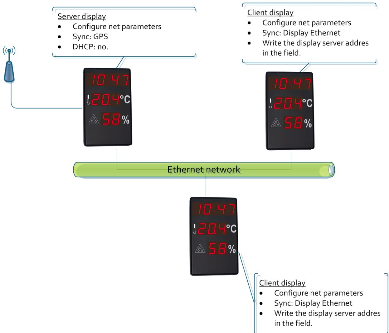
**Sync through SNTP. Only one display connects to the SNTP server.**
