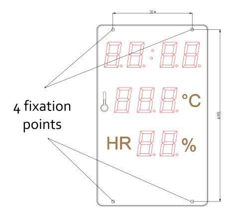
The DC-41 SRTHNE+2R/+4R displays can be fixed to the wall in two ways:
