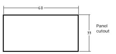
Min. thickness : 0.8mm Max. thickness : 10mm
