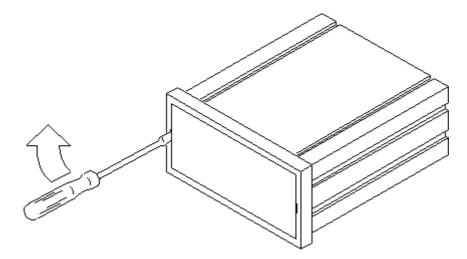
Remove lens by placing an appropriate sized screwdriver in the slot and pushing laterally until the lips disengange. Unscrew the rear nut to lift the circuits out from the front of the case. To reinstall lens, insert it completely from one side and press from the other until it is perfectly fitted.
