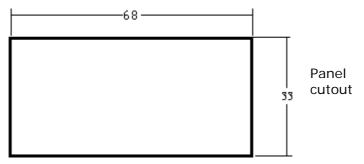
Min. thickness : 0.8mm Max. thickness : 10mm
