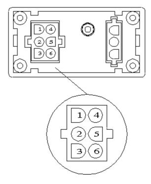
Input signal PIN 1 Spare PIN 2 Input signal (+) PIN 3 Input signal (-)
