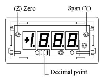
The frontal lens are removable to provide access to zero, span adjust and to decimal point location.
