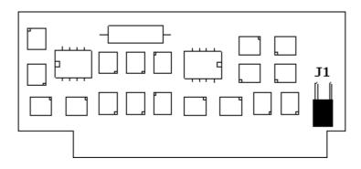
To change the scale, place internal jumper J1 as indicated below and locate the decimal point to the proper position.
