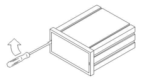
Remove lens by placing an appropriate sized screwdriver in the slot and pushing laterally as it is shown in the figure until the lips disengange.
