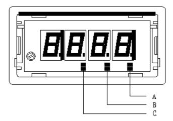
To change the decimal point location, remove the frontal lens and solder the appropriate jumper as indicated here below:
