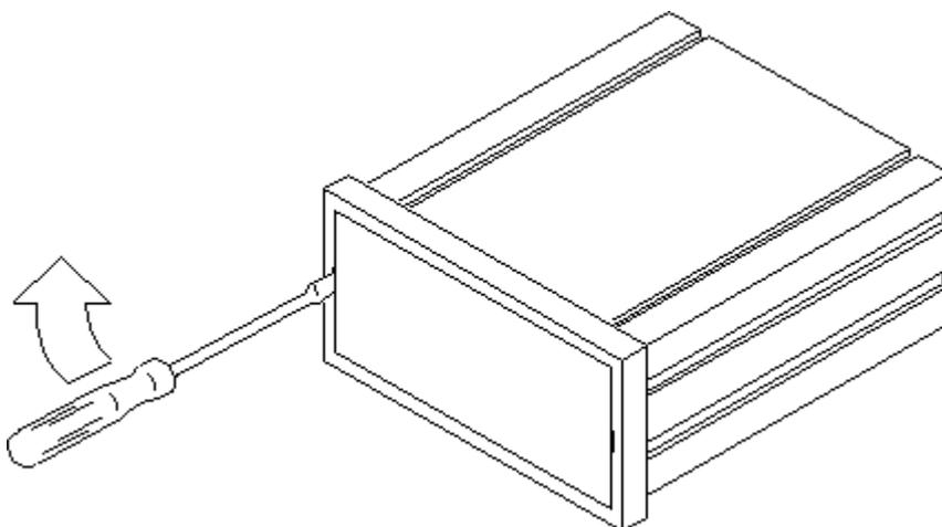
Remove lens by placing an appropriate sized screwdriver in the slot and
