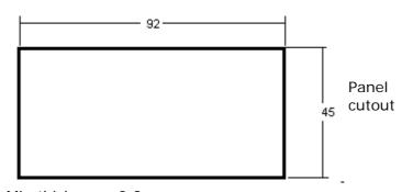
Min.thickness: 0.8mm Max.thickness: 10mm
