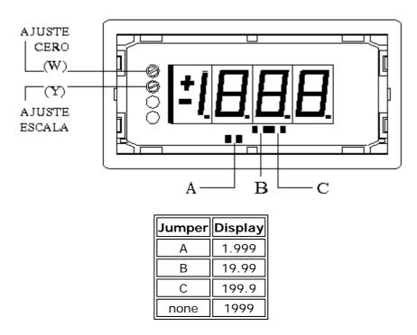
The **zero adjust** corresponds to the potentiometer (W) located to the upper, left side of the display. Turning clockwise decreases the display reading. The adjustment margin is  $\pm 200$  counts.
