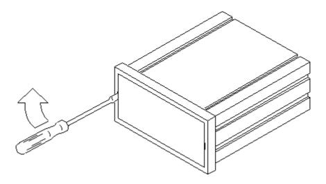
Remove lens by placing an appropriate sized screwdriver in the slot and pushing laterally as it is shown in the figure until the lips disengange. For further configuration unscrew the rear nut to take the circuits out from the front of the case.
