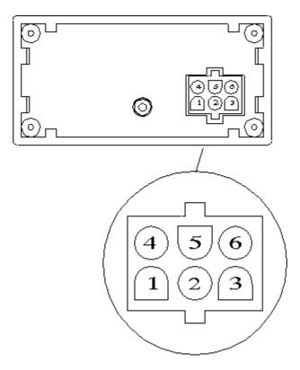
Input signal PIN 1 Spare PIN 2 AC input signal PIN 3 AC input signal PIN 5 Spare
