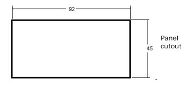
Min. thickness: 0.8mm Max. thickness: 10mm
