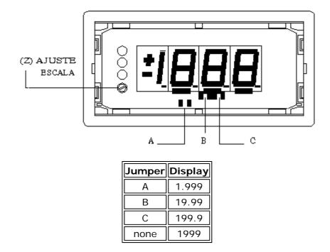
The **span adjustment** is made by the potentiometer (Z) located to the left, lower side of the display. Turning clockwise increases the display reading. The adjust margin is  $\pm$  20% of F.S.
