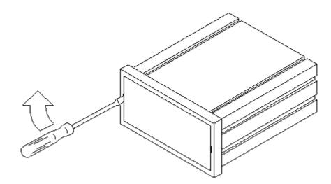
Remove lens by placing an appropriate sized screwdriver in the slot and pushing laterally as it is shown in the figure until the lips disengange. For further configuration unscrew the rear nut to take the circuits out from the front of the case.
