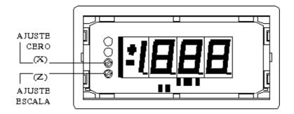
**Cold-junction compensation:** Shortcircuit pins 2 and 3 at the connector and adjust the zero potentiometer until the display reads the ambient temperature.
