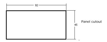
Min. thickness: 0.8mm Max. thickness: 10mm
