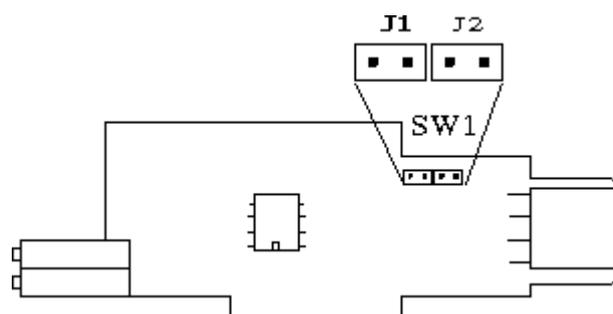
In order to compensate the resistance contributed by the zener barrier, plug in the jumper of group SW1 according to the following table:
