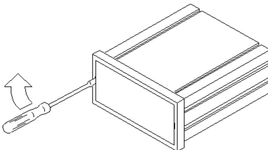
Remove lens by placing an appropriate sized screwdriver in the slot and pushing laterally as it is shown in the figure until the lips disengage.
