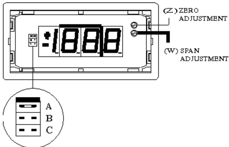
The zero and span adjust is made by the potentiometers (Z) and (W) respectively, located to the upper right side of the display.
