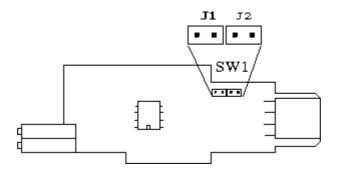
In order to compensate the resitance contributed by the zener barrier, plug in the jumper of group SW1 according to the following table:
