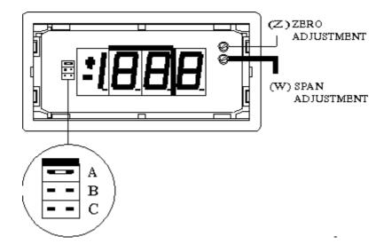
The zero and span adjust is made by the potentiometers (Z) and (W) respectively, located to the upper right side of the display.
