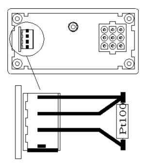
3-wire connectivity PIN A Pt100 PIN B Pt100 PIN C common Pt100 PIN D Spare
