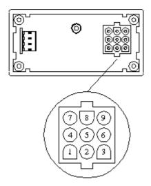
AC power supply PIN 7 AC HI PIN 9 AC LO (neutral)
