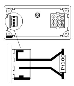
2-wire connection Tie pins A and B toghether at the connector. Connect the Pt100 between pins C and B.
