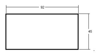
Panel cutout Min. thickness: 0.8mm Max. thickness: 10mm
