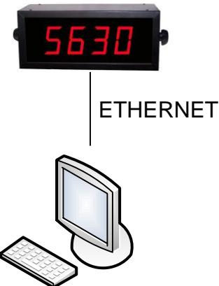
To connect various displays, a switch type concentrator or hub must be used with a port for each unit.
