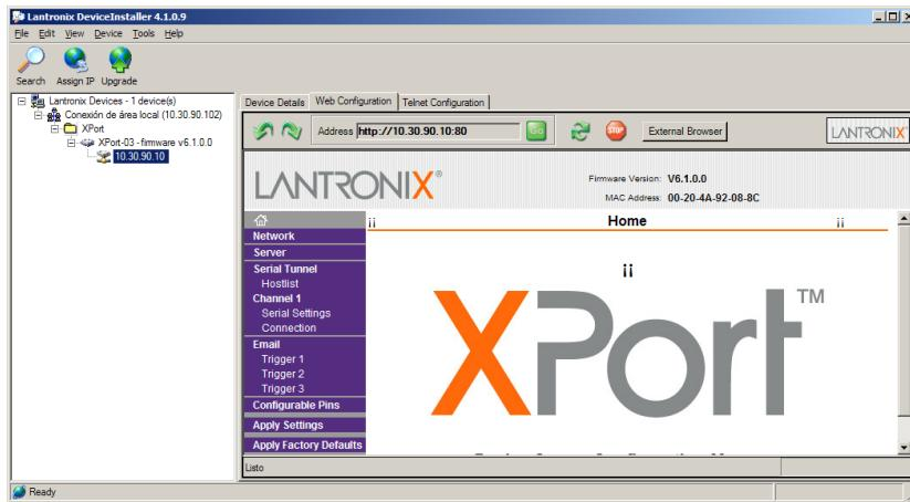
To access the setup the Local Port, select **Channel1->Connection**.
