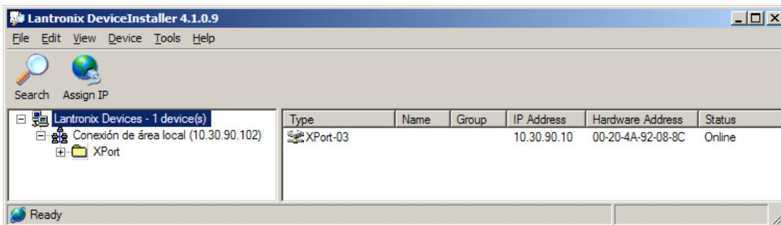
The IP address with which the equipment is supplied is: 10.30.90.10
