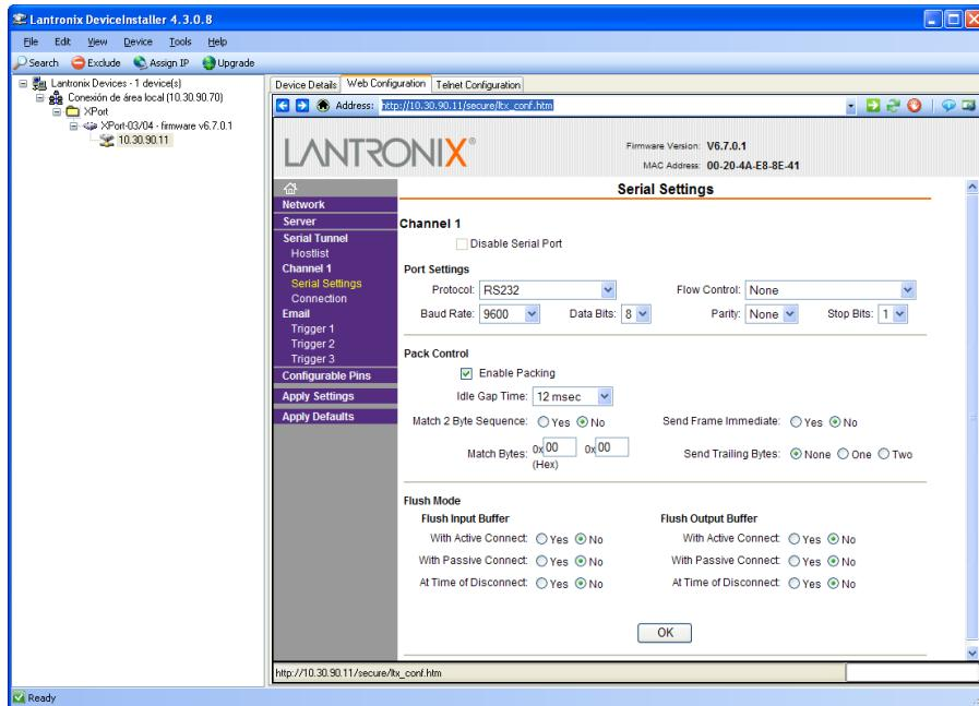
In order to check **Enable Packing** bit setting you must exit the Web Configuration page and re-enter. Click **Search** on menu and enter again into the Web Configuration.
