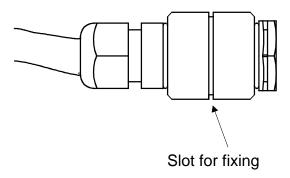
In order to attach it, a clip-type base is supplied. In order to open it, introduce a flat screwdriver through the slot market «Open» and press slightly outwards and pull upwards. Once you have attached the base, place the sensor on the clip in such a way that the slot of the sensor coincides with the protection of the clip. Close the clip and you will have the sensor in place.
