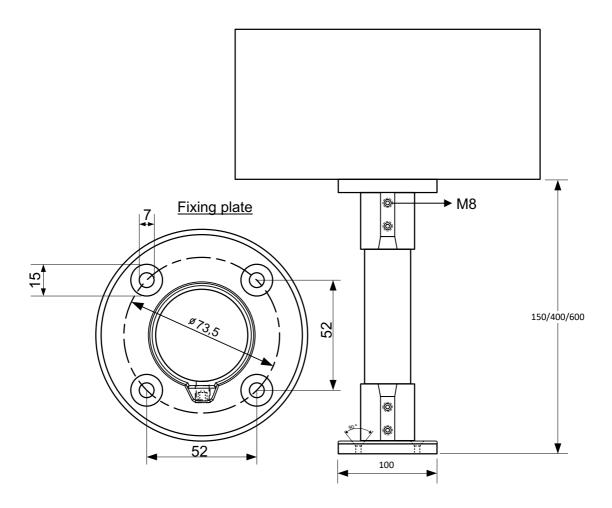
All the measurements are in millimeters
