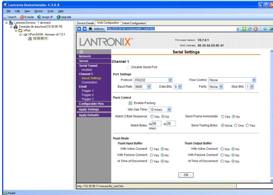
In order to check **Enable Packing** bit setting, you must exit the Web Configuration page and re-enter. Click **Search** on the menu and enter again into the Web Configuration.
