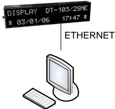
To connect various displays, a switch type concentrator or hub must be used with a port for each unit.
