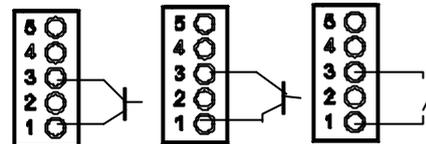
Figure. 29.2 Connection examples. PNP, NPN or switch.
