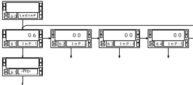
The logical functions are programmed on module '60 LoGInP'. There are 4 menu every one of them corresponds to one input on connector CN2:
