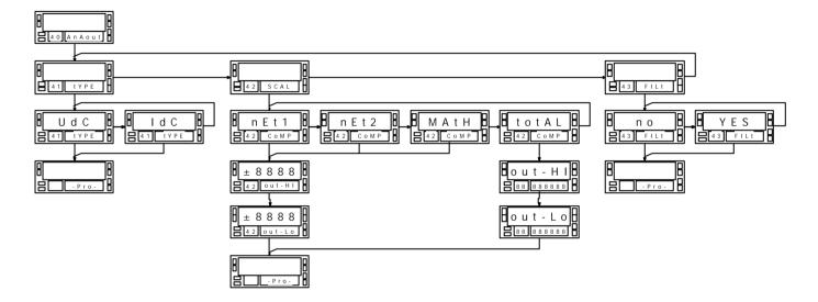
The analog output is refreshed every 10 mS. The analog output should be related to any display range and be selected to work with Net1, Net2, Math or TOTAL (whenever t his variable is authorized)
