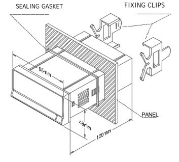
Place the fixing clips on both sides of the case and slide them over the guide tracks until they touch the panel at the rear side.
