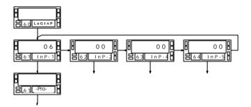
The logical functions are programmed on module '**60 LoGInP**'. There are 4 menu every one of them corresponds to one input on connector CN2: 61 InP-1: Input pin 1 62 InP-2: Input pin 2 63 InP-4: Input pin 4 64 InP-5: Input pin 5 The pin 3 is the common.
