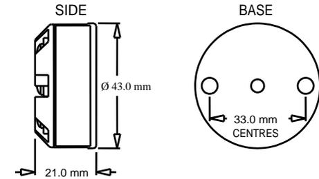
Mounting holes: two holes 5.5mm diameter, 33mm centres
