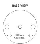
Fixing holes 2 x Ø5.5 mm Centre hole Ø4.0 mm
