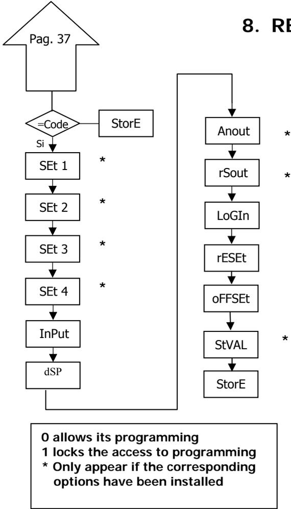
Following the herewith diagram, factory configuration can be restored:
