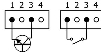
The external electronics applied to the CN3 connector must be capable of withstanding 40 V and 20 mA present at all terminals with respect to COMMON. In order to guarantee the electromagnetic compatibility, please refer to the instructions given on page 9.
