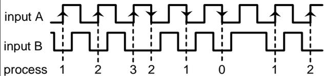
**Programming diagram of the DISPLAY in MODE: COUNTER**
