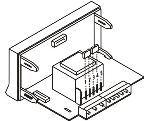
Fig. 9.3. Jumper settings for 115 V or 24 V AC
