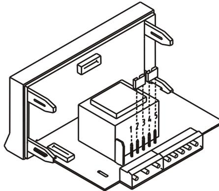
Fig. 9.2. Jumper settings for 230 V or 48 V AC
