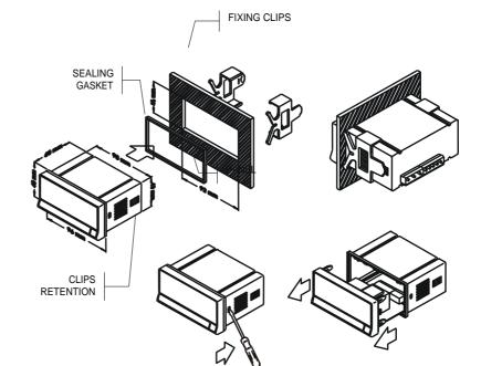
Place the fixing clips on both sides of the case and slide them over the guide tracks until they touch the panel at the rear side. Press slightly to fasten the bezel to the panel and secure the clips.
