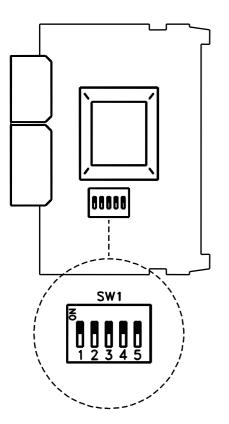
Before undertaking signal connection, set the input for the sensor type to be used in the application by means of the SW1 5-position DIP switch located on the main board.
