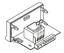
Fig. 9.3. Jumper settings for 115 V or 24 V AC
