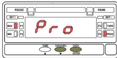
The figure 15.1 represents the entry level of the input configuration module (**Pro** indication, **F1** and **PROG** LED's activated).
