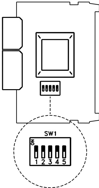
Before undertaking signal connection, set the input for the sensor type to be used in the application by means of the SW1 5-position DIP switch located on the main board.
