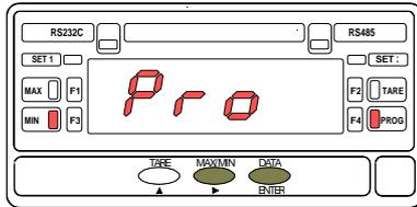
The figure 21.1 represents the entry level of the display configuration module (**F3** and **PROG** LEDs activated). Press **ENTER** to access this module. After the programming has been completed, the instrument will return to this stage. From here, to go to the normal operation, press **▶** as many times as to deactivate all the functions LED's except the PROG one and press **ENTER** to store changes in the memory and exit from the program routines.
