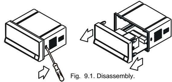
Fig. 9.1. Disassembly.
