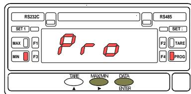
The figure 19.1 represents the entry stage of the display configuration module (**F3** and **PROG** LED activated). Press **ENTER** to access this module.
