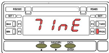
The sampling time (see page 19), two digits with decimal point, appears on the display after the symbol shown in the left figure.
