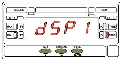
After programming the input frequency, a press of **ENTER** provides access to the programming of the display desired for this frequency (**dSP1**), preceded by the symbol shown in figure 20.1. Proceed as in the section 19.3. (**▲** increments value, **▶** advances to the next digit) to compose the desired value and press to set the decimal point position (by means of the **▶** key). Press again **ENTER** to exit from the program module and return to the **Pro** stage shown in fig. 19.1.
