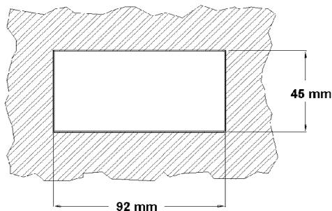
Place the fixing clips on both sides of the case and slide them over the guide tracks until they touch the panel at the rear side. Press slightly to fasten the bezel to the panel and secure the clips.
