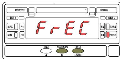
The display presents the initially selected input type : **FrEC** = FREQUENCY METER, **TAC** = TACHOMETER, **rATE** = RATE METER. Press repeatedly the **▶** key to scroll around the available options until the desired one appears on the display and press **ENTER** to validate the choice and automatically return to the **Pro** stage indicated in the figure 15.1.
