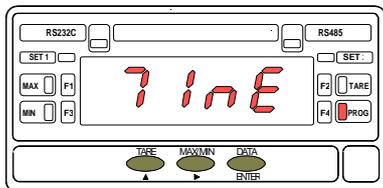
The sampling time (see page 17), two digits with decimal point, appears on the display after the symbol shown in the left figure. Make use of the **▲** and **▶** procedure if wanted to modify the initially programmed value (from 1.0 to 9.9 seconds) and press **ENTER** to save the entry in the memory and to access to the programming of the limit time.
