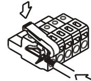
Proceed in the same manner with all pins and plug the terminal block back to the corresponding meter's connector.
