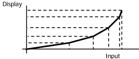
In order to obtain more accuracy in the measuring it is recommended to program the highest possible number of points and reduce the segment length.
