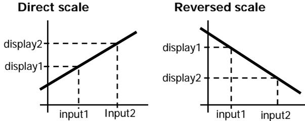
**In linear processes** it is achieved by programming two coordinates (input1, display1) and (input2, display2), between which is established a linear relation where to each input signal value corresponds a display value. The relationship can be direct or reversed. In order to obtain more accuracy, points 1 and 2 should be located approximately at both extremes of the process.
