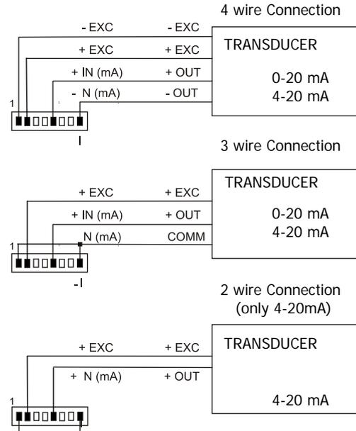
If the excitation supplied by MICRA-M to the transducer has to be 10 or 5 V connect the + EXC wire to PIN3 instead of PIN2
