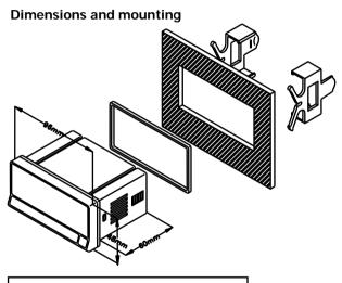
Front: 96 x 48 mm Depth: 60 mm Panel cut-out: 92 x 45 mm
