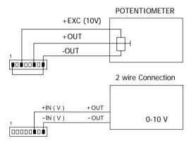
If the excitation supplied by MICRA-M to the transducer has to be 10 or 5 V connect the + EXC wire to PIN3 instead of PIN2
