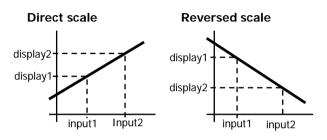
In linear processes it is achieved by programming two coordinates (input1, display1) and (input2, display2), between which is established a linear relation where to each input signal value corresponds a display value. The relationship can be direct or reversed. In order to obtain more accuracy, points 1 and 2 should be located approximately at both extremes of the process.
