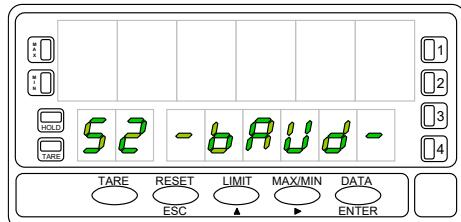
An "ENTER" in the previous step makes the initially programmed baud rate appear on the main display.
