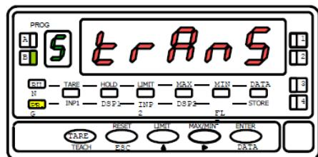
A flashing number appears on the display (1,2 or 3 depending on the previous selection) corresponding to the current communication protocol
