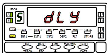
An in the previous step, it flashes a number (between 1 and 4 according to previous programming) on the display [**1** = 30ms delay, **2** = 60ms delay
