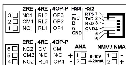
Each output card is supplied with an adhesive label indicating the connection of each of the options.
