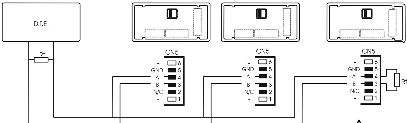
Up to 31 DITEL indicators can be connected on the same line with a D.T.E. by assigning each of them a unique address between 00 and 99.
