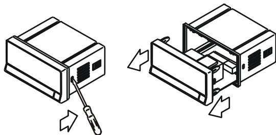
Extract the electronic assembly from the box and break the joints in the gray area of the figure to separate it from the box.
